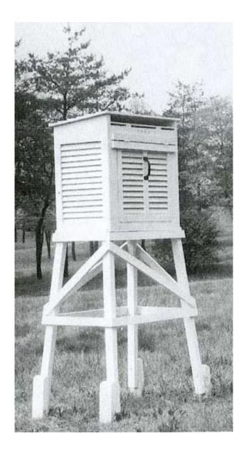
Figure 21. Cotton Region Instrument Shelter of a Type Used in Milwaukee Source: National Archives and Records Administration
