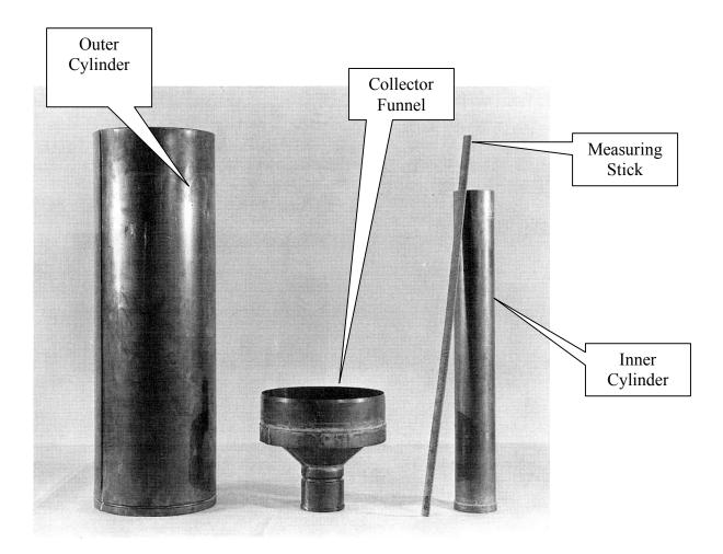
Figure 17. Standard Eight Inch Rain Gauge Source: National Archives and Records Administration In 1899, the rain gauge stood near the middle of the roof on the Federal Building about 116 feet above ground level. There were no obstructions that interfered with the catch.
