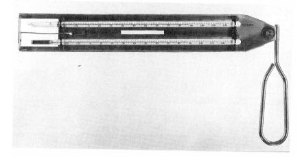
Figure 15. Sling Psychrometer, Wet Bulb above, Dry Bulb Below Source: National Archives and Records Administration
