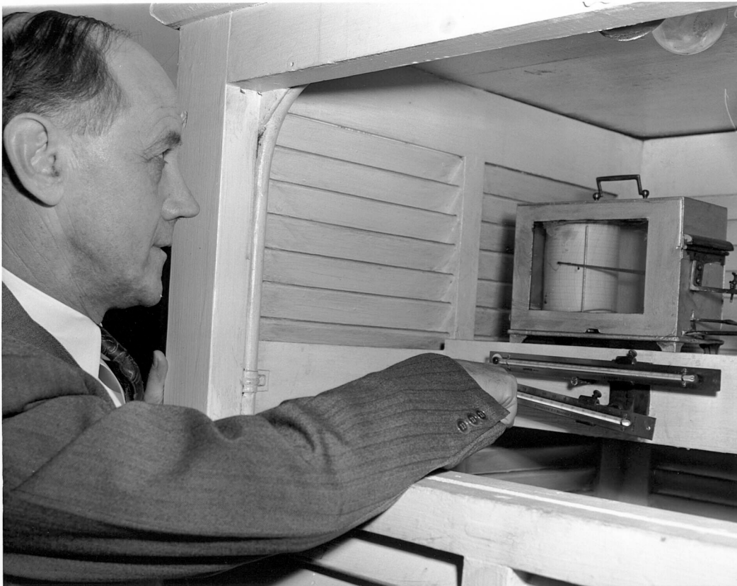
Figure 13. Maximum (below) and Minimum (above) Thermometers, 1960 Source: Seattle Museum of History and Industry, Seattle Post-Intelligencer Collection
