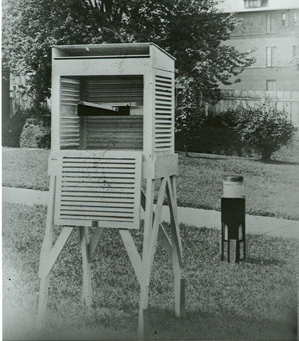
Figure 32. Maximum and Minimum Thermometers In the Instrument Shelter Source: Utah Historical Society, J. Cecil Alter Collection, C-102 Box 1
