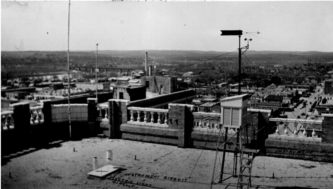
Figure 10. The suite of weather observing instruments on the roof of the Littlefield Building in Austin, Texas, as of March 1932. View is looking west northwest. Source: Official station history files at the National Climatic Data Center.
