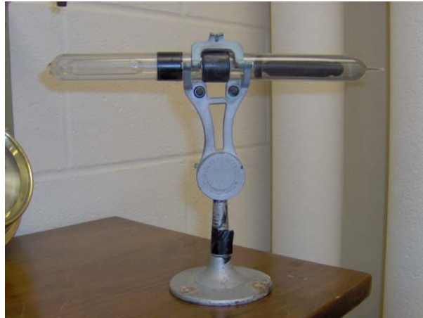
Figure 24. Sunshine Recorder, College Heights Weather Station Museum Source: Author
