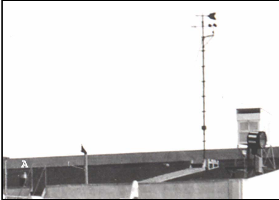
Figure 12. Enlargement of photograph in Figure 10 showing Weather Bureau instrument shelter, wind instruments, and rain gage (located in the lower left hand part of the photograph directly below point “A”). View is southeast. From the Oregon Historical Society.
