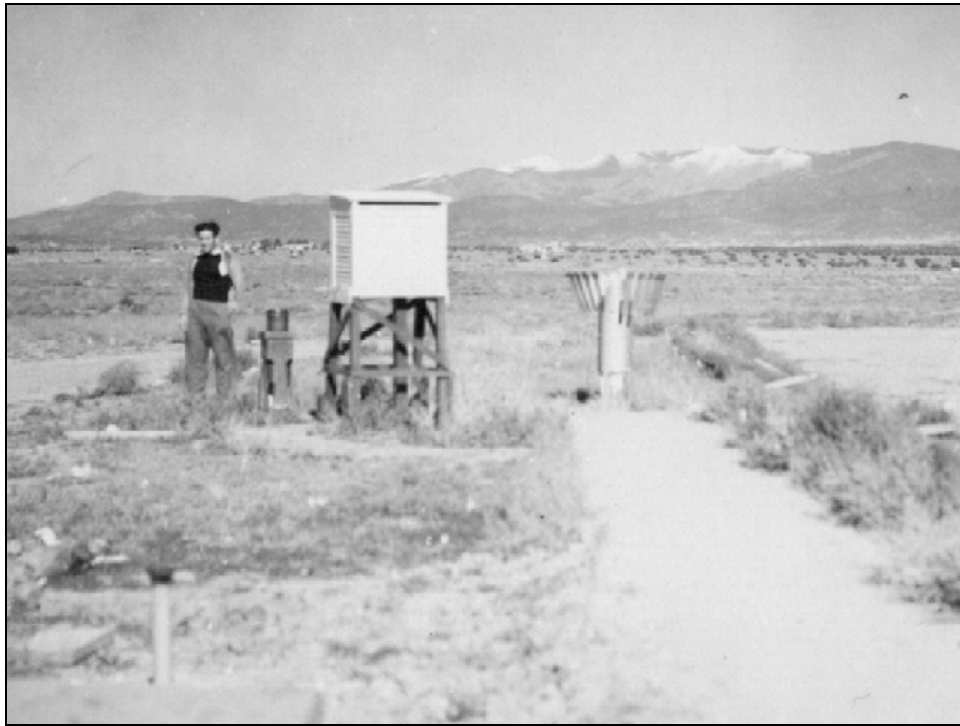
Figure 20. Instrument shelter and rain/snow gages. View toward north northeast from the Administration and Hanger Building at the old Santa Fe Airport. Picture taken Oct 1942. From the official station history files at the National Climate Data Center.
