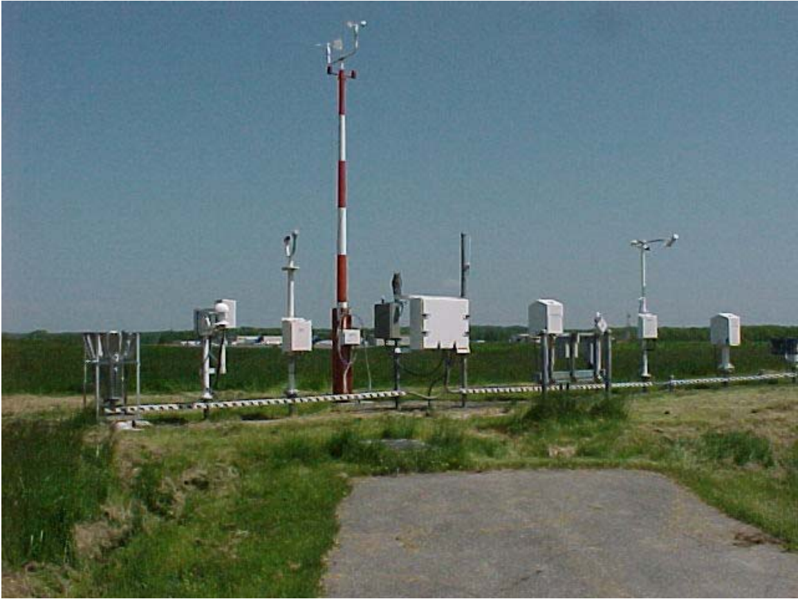
Figure 19. The ASOS instrument suite at the Portland International Jetport in 2004. From the Gray, Maine office of the National Weather Service.
