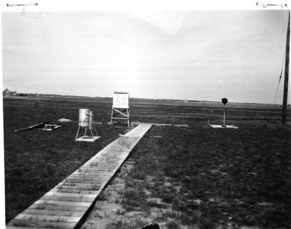
Figure 16. A view of the instrument shelter and rain gages at the Nantucket, Massachusetts, Memorial Airport on May 9, 1946. Original caption read “View looking North-east showing instrumental equipment.” From the Station History files at the National Climatic Data Center.
