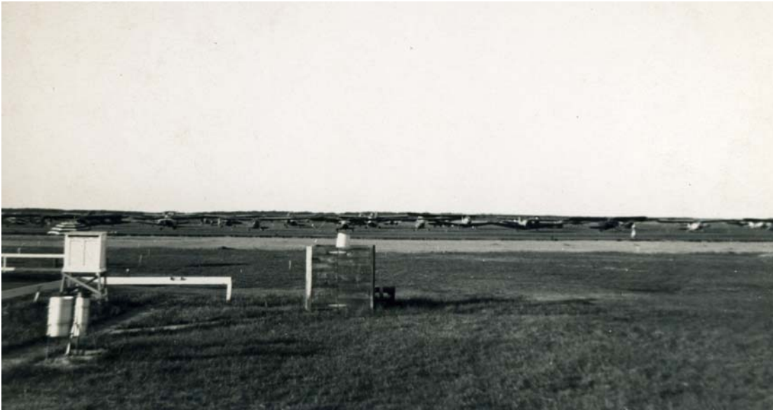
Figure 18. Weather instruments located at the Memorial Airport, Nantucket, Massachusetts in 1949. Notice the instrument shelter to the left rear and the rain gages to the left front. The direction of the view is unknown. Photograph from the Nantucket Historical Association (PH2-3-14).
