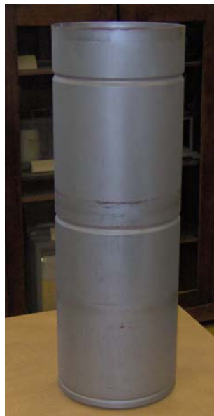
Figure 15. Standard 8 Inch Rain Gage, College Heights Weather Station, used 1928 to 1965 Source: Author
