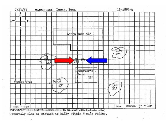
Figure 9. The location of instruments at Logan, Iowa, on 27 July 1973. The red arrow points to the location of the Cotton Region Shelter, while the blue arrow indicates the location of the rain gage.
