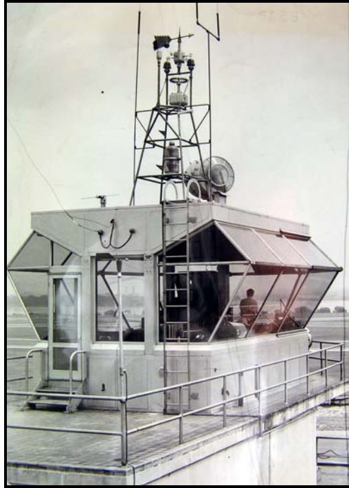
Figure 15. Wind instruments over tower of National Airport (circa late 1940s). Anemometer is located to the immediate left of the wind vane with anemometer cups obscured by the tail of the wind vane. From the Martin Luther King Jr. Memorial Library.
