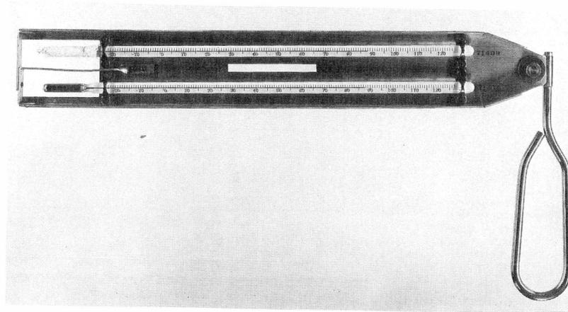
**Figure 15. Sling Psychrometer, Wet Bulb above, Dry Bulb Below**
