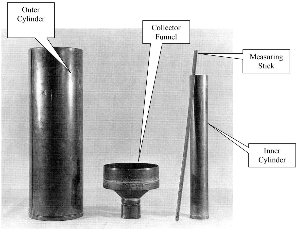
**Figure 17. Standard Eight Inch Rain Gauge**
