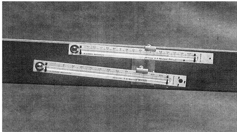
**Figure 14. Green Maximum and Minimum Thermometers**
