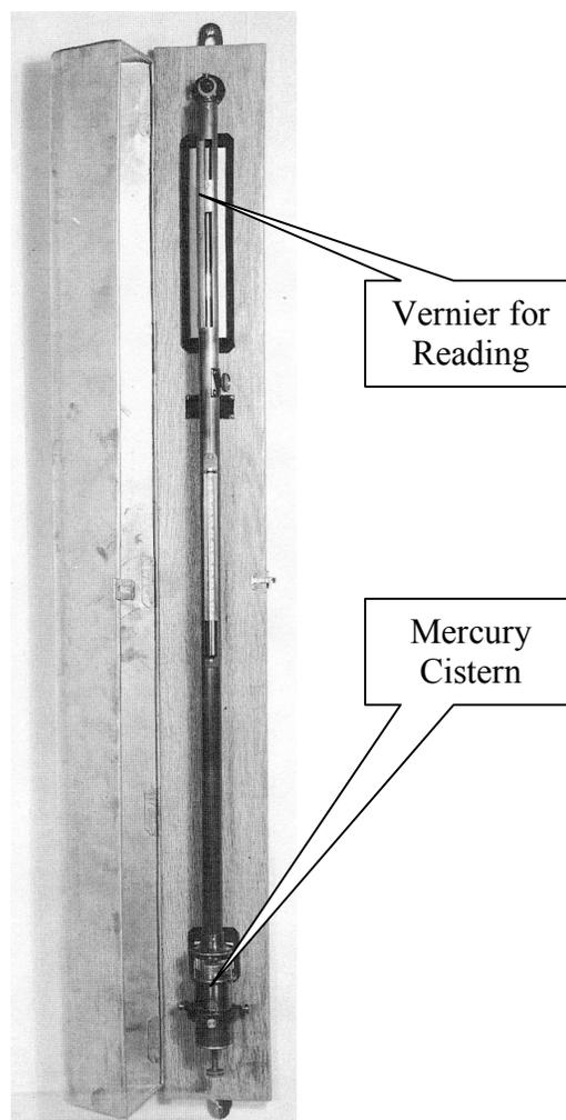
**Figure 18. Mercury Barometer**
