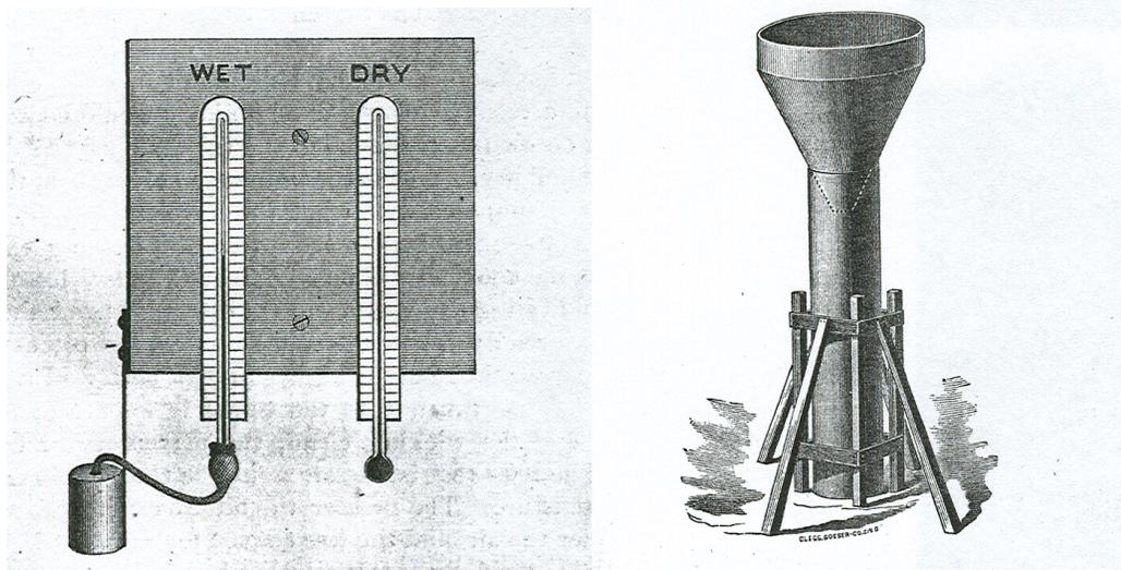
**Figure 14. Hygrometer and Rain Gauge for Sale circa 1883**
