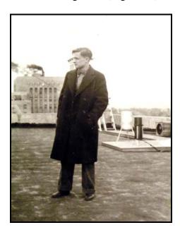
Figure 13. Tipping bucket and standard eight-inch rain gage on top of the Kimo Theatre Building (circa 1932). View is toward the south. Person in the picture was a Weather Bureau employee. From the files of the National Weather Service Forecast Office in Albuquerque, NM.
