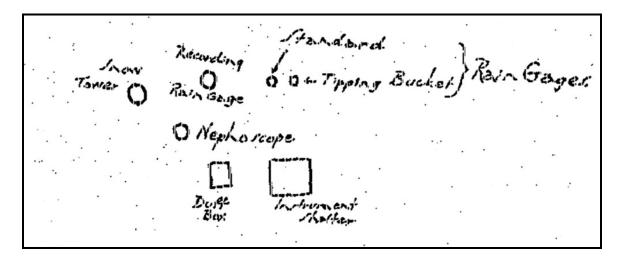
Figure 20. Arrangement of weather instruments near the Municipal Airport Administration Building (6 September 1943). Arrangement is representative (with the exception of the weighing, or recording rain gage that was added in late 1940 or early 1941) through the 1940s. North is to the left. From the official station history files at the National Climatic Data Center.
