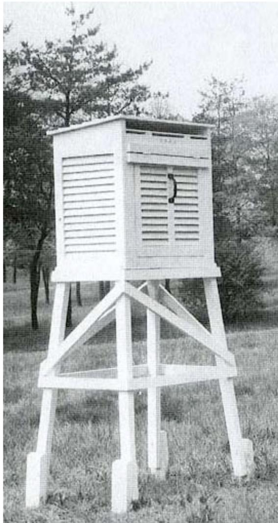
**Figure 27. Cotton Region Instrument Shelter of a Type Used in Helena**
