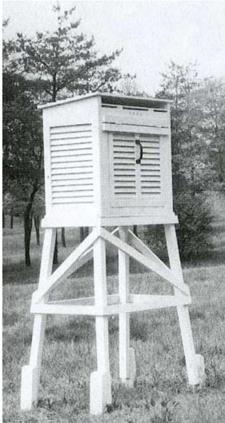
**Figure 16. Cotton Region Instrument Shelter was the Type Used in Sonoma**
