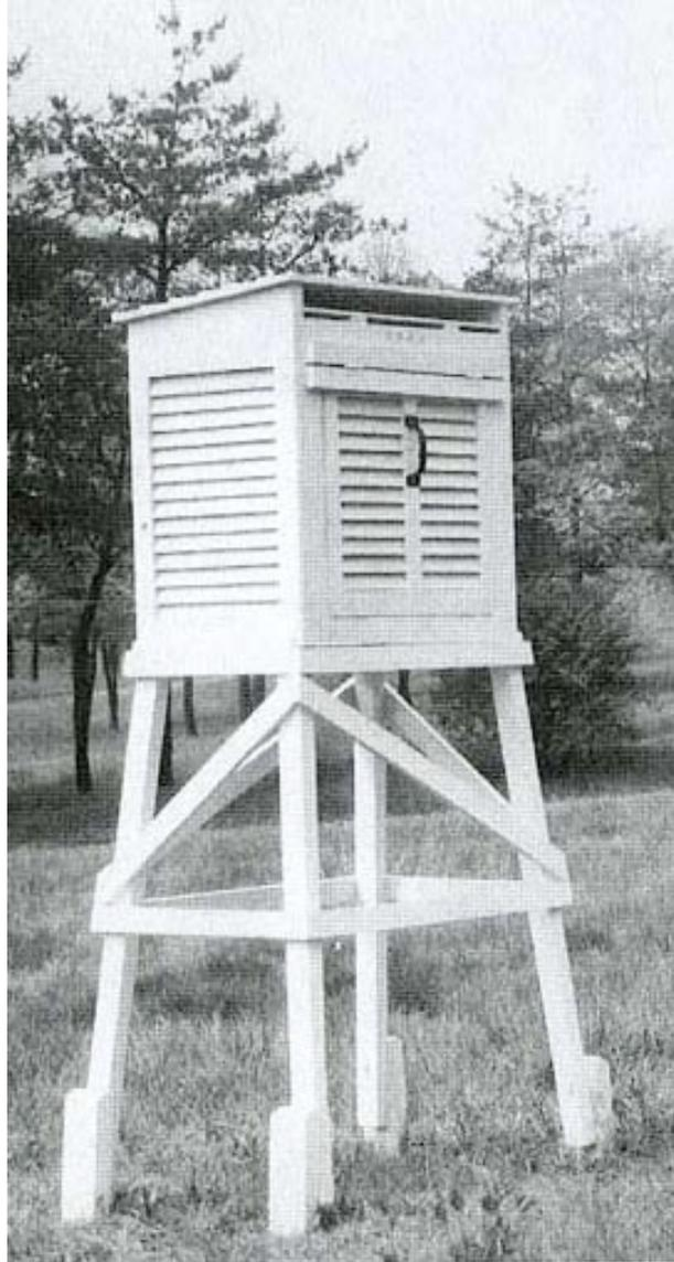
**Figure 16. Cotton Region Instrument Shelter of a Type Used in Wickenburg**
