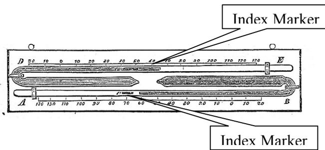
**Figure 9. Self-Registering Thermometer**
