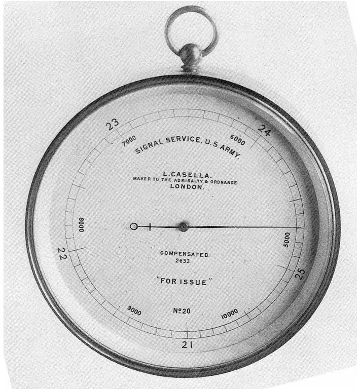
**Figure 17. Signal Service Type 1 Aneroid Barometer**
