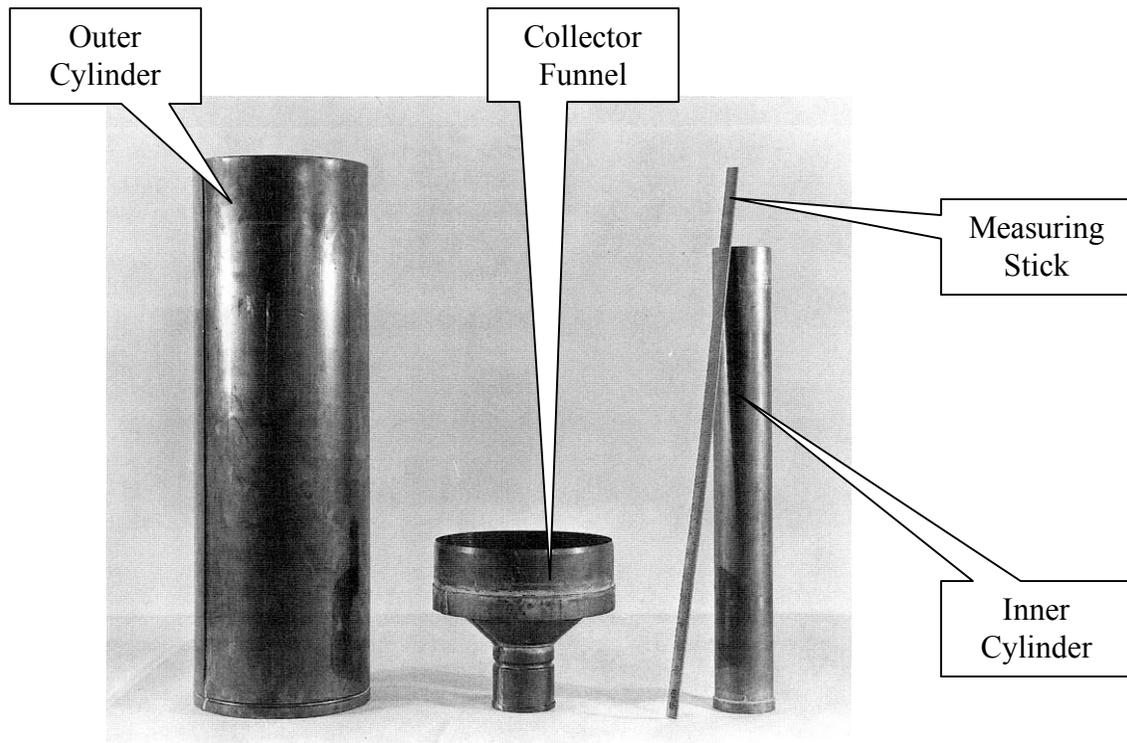
**Figure 14. Standard Eight Inch Rain Gauge**
