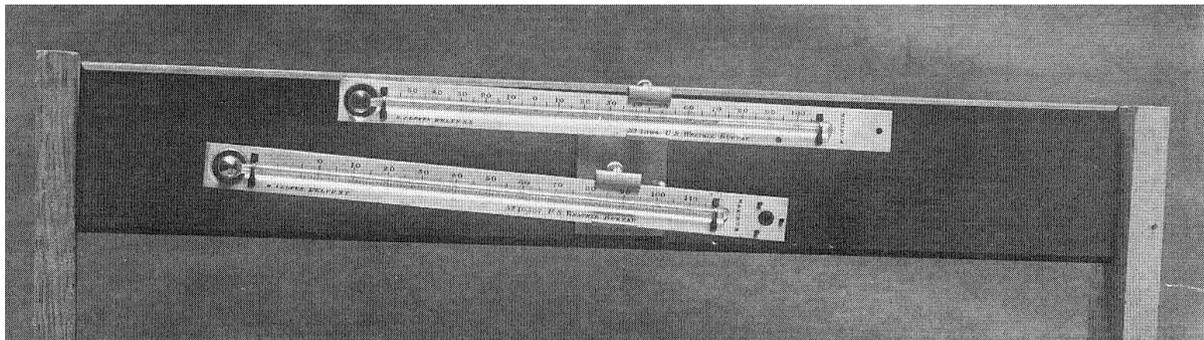
**Figure 10. Green Maximum and Minimum Thermometers on a Townsend Mount**
