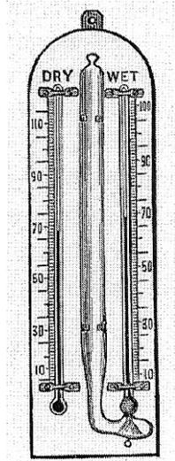
**Figure 16. Mason's Hygrometer, 1879**
