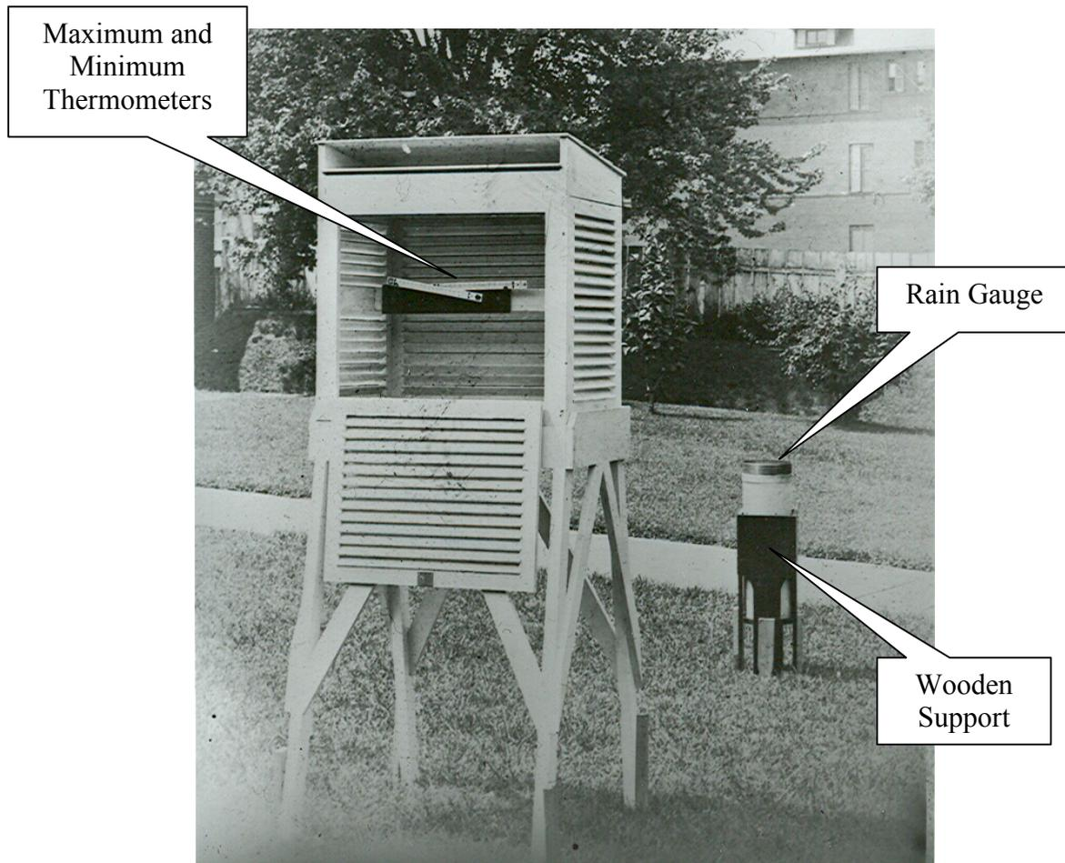
**Figure 15. Maximum-Minimum Thermometers in Instrument Shelter, Rain Gauge on Right**
