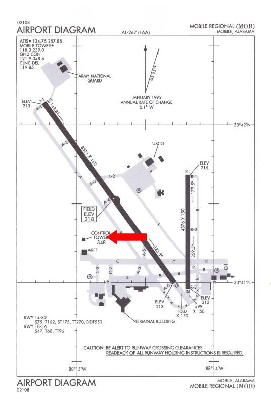
Figure 22. A diagram of the Mobile Regional Airport, 1995. The red arrow indicates the location of the ASOS weather instruments. Source: Authors personnel collection of airport diagrams.
