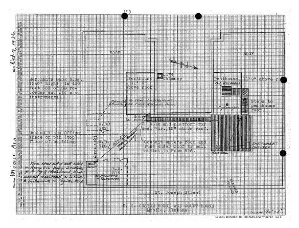
Figure 10 The layout of the weather instruments in October 1936 located on the roof of the U. S. Court House and Customs House in Mobile, Alabama. Source: Official station history files at the National Climatic Data Center.
